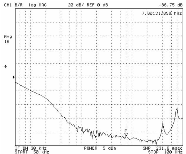
Fig. 4: Common Mode attenuation, 0.05-100 MHz. Source and load resistances are 50 Ω. Two 0.47 µF Y-caps to common line. Vertical scale: 20 dB/div, with zero dB level marked by arrow.
